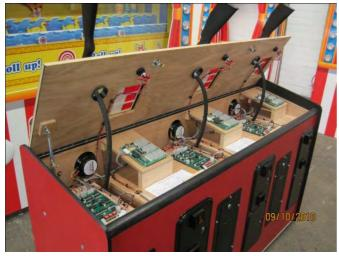
Coin doors – Opening the top door gives access to the coin mechanism, and opening the bottom door gives access to the cash box.
