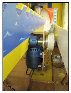
The profile ducks are fastened to a toothed timing belt,
